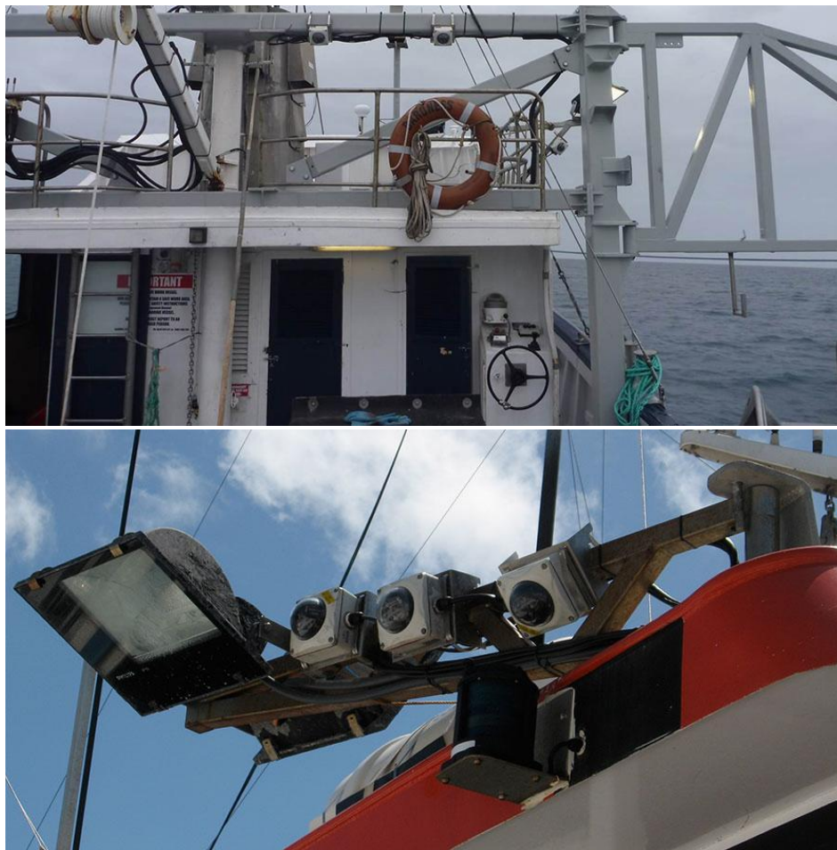
Figure 18. AFMA Electronic Monitoring System installed on a boat
