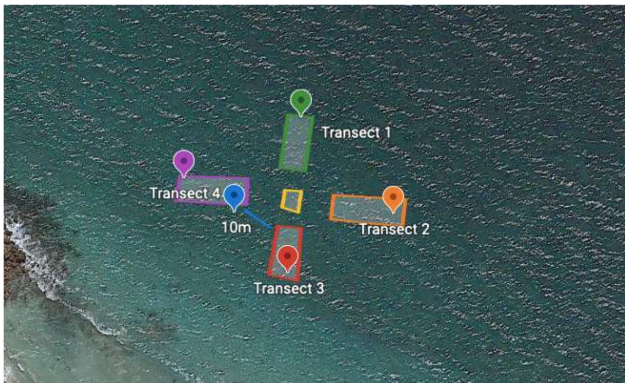
Image 5.12 - Transects are set at 90 degree intervals around the boat, forming a cross shape*.
