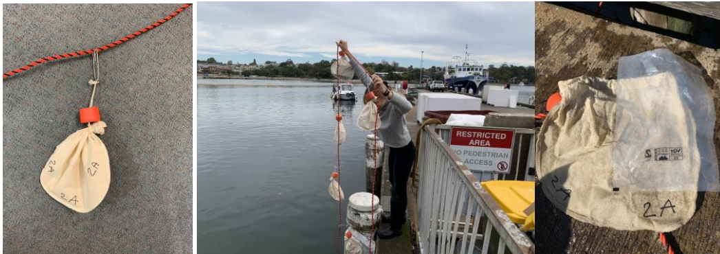
Figure 18. Alternative packagings were placed in cotton bag and emerged in seawater in Pymont, NSW
