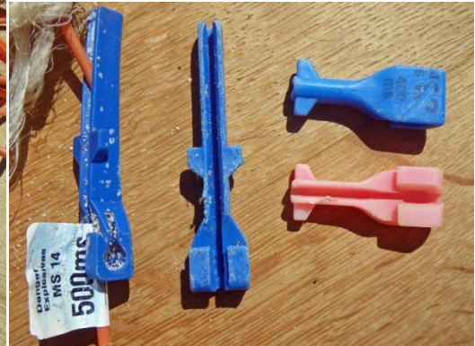
Red Cord (Detonator Shock Tube) with Clip is shown at left with an assortment of clips shown below
